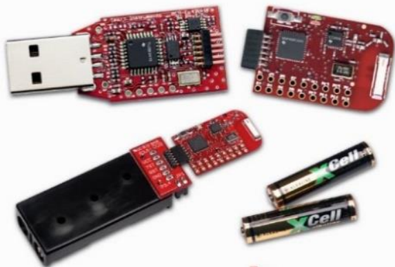
Fig. 3. Kit de dezvoltare wireless front end eZ430-RF2500 microcontroler si transceiver wireless
