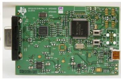
Fig. 3. AFE4400 SpO2 and HR evaluation module
